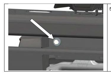
5. Secure Top mounts using the bolt lengths and or washers shown below.
